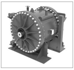
SONDEX<sup>®</sup> Spiral heat exchangers are exceptionally well-suited for sludges, slurries, waste water, liquids with high viscosity, and liquids that contain fibers and solids. SONDEX<sup>®</sup> spiral heat exchangers are the definitive solution for applications that require treatment of challenging fluids. The design allows for a countercurrent flow that makes it possible to achieve close temperature approaches.
